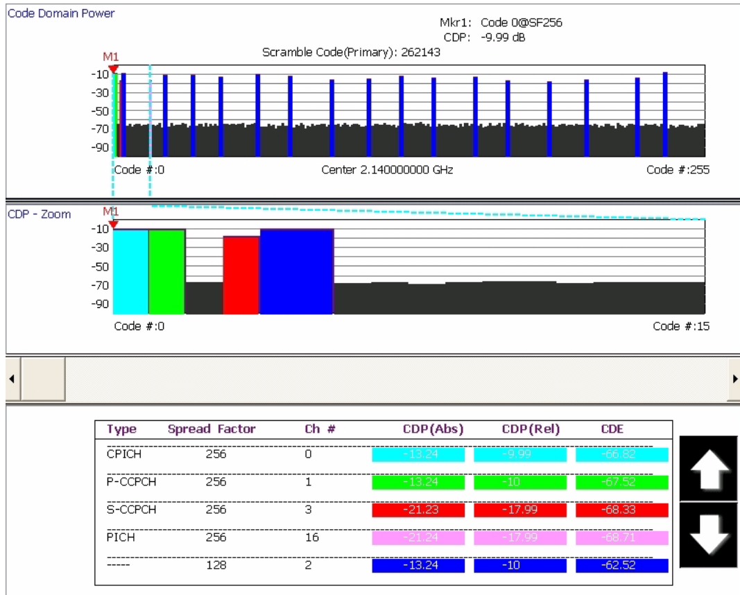
Figure 6-24. Code Domain Power for Test Model 1 with Zoom and Summary Table
